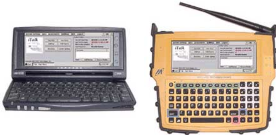
The iTalk™ rapid damage assessment application running on HP Jornada™ and SideArm™ handheld PCs.
